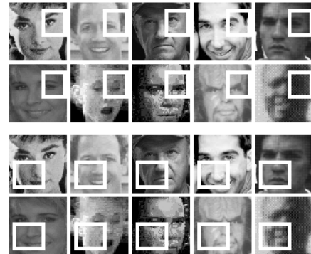
Fig. 1: The first and second covariance region selected by AdaBoost. The figure displays the first two covariance features overlaid on human faces. The first covariance feature captures the information of the right eye while the second covariance feature describes the contour of the face, and the region around the nose.
